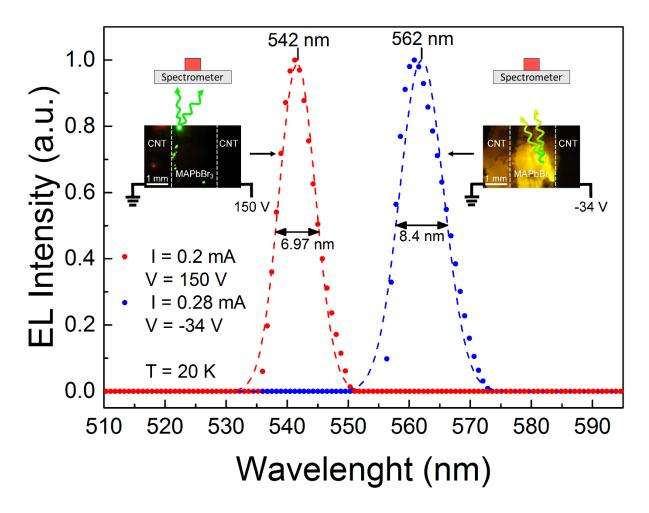
**Figure 4.** The typical normalized EL spectra recorded at 20 K in vacuum, at positive (red, +150 V) and negative (blue, -34 V) bias voltages, fitted with Gaussian function (dashed lines). Inset: Schematic illustration of the measurement setup with the photos of the light emission for the associated EL spectra.
