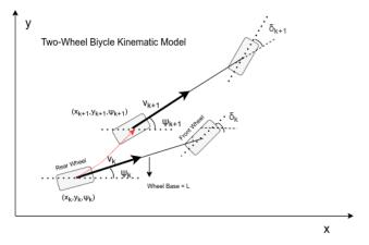
Fig. 3: Kinematics model of the control algorithm
