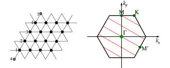
FIG. 1: Left panel: Triangular lattice on a cylinder with  $L_2 = 4$ , with periodic boundary conditions along  $\mathbf{a}_1$  and  $\mathbf{a}_2$ . This geometry is different from the YC4 one of Refs. [38, 39]. Right panel: First Brillouin zone of the triangular lattice. The red dashed lines indicate the allowed momenta on a cylinder with  $L_2 = 4$ .
