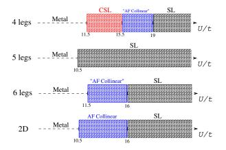
FIG. 7: Schematic phase diagram of the triangular lattice at t'/t = -0.3, as a function of U/t. Four different lattices are considered, with 4, 5, and 6 legs, as well as a two dimensional cluster. The symbol "SL" denotes a gapless spin liquid, while the symbol "CSL" denotes a chiral gapped spin liquid. The antiferromagnetic collinear order on cylindrical geometries is denoted in quotation marks, since no true long-range magnetic order can occur.
