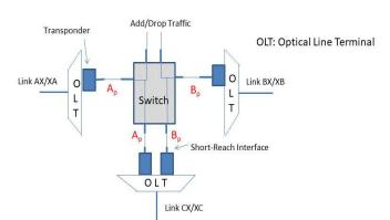
Fig. 2. Optical Node X in Opaque Architecture Without Network Coding
