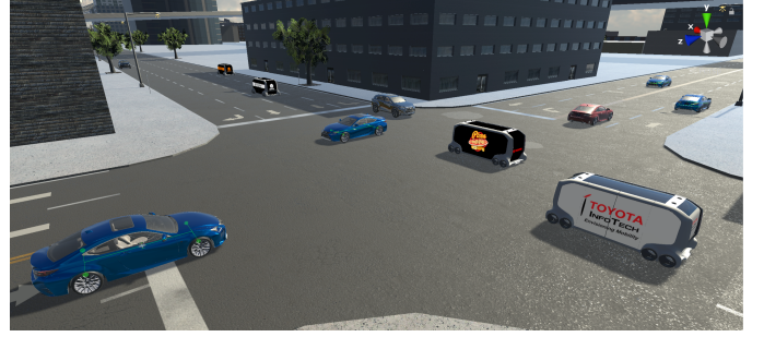
Fig. 8. A snapshot of the Unity simulation, where connected vehicles cooperate with each other at a non-signalized intersection
