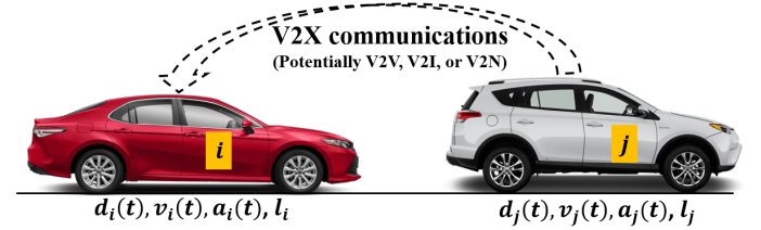
Fig. 3. The illustration of vehicle parameters in a V2X communication environment with an ego vehicle i and its target vehicle j
