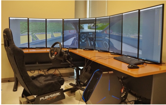
Fig. 7. Driving simulator platform to conduct human-in-the-loop (HITL) simulation
