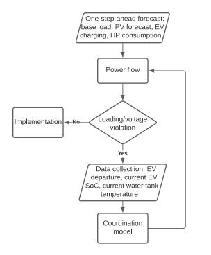
Fig. 1. Real-time operation procedure
