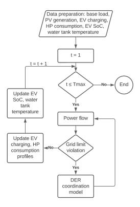
Fig. 4. Simulation flowchart
