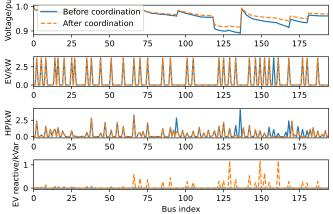
Fig. 7. Voltage magnitude, EV/HP power and EV reactive power generation for a time slot
