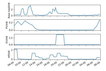
Fig. 3. Base load, PV, EV, HP profiles for a household for the selected day, starting from 8:00 with a 15-minute resolution
