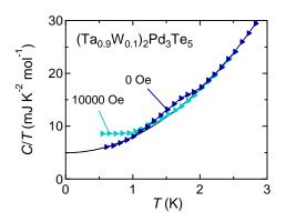
Supplementary Fig. 5. Temperature dependence of the heat capacity divided by the temperature of the  $(Ta_{0.9}W_{0.1})_2Pd_3Te_5$  polycrystalline sample measured under a zero magnetic field and 10000 Oe. The solid curve shows a fit of the equation  $C/T = AT^2 + \gamma$ , yielding A = 3.00(3) mJ K<sup>-4</sup> mol<sup>-1</sup> and  $\gamma = 4.96(13)$  mJ K<sup>-2</sup> mol<sup>-1</sup>.
