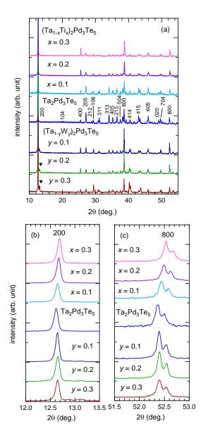
Supplementary Fig. 2. Powder XRD patterns (a) and those around the 200 (b) and 800 (c) reflection peaks of the  $(Ta_{1-x}Ti_x)_2Pd_3Te_5 (x = 0.1, 0.2, and 0.3)$  and  $(Ta_{1-y}W_y)_2Pd_3Te_5 (y = 0.1, 0.2, and 0.3)$  polycrystalline samples measured at room temperature. The data of undoped Ta<sub>2</sub>Pd<sub>3</sub>Te<sub>5</sub> presented in Fig. 1(c) are also shown as a reference. The peaks indicated by triangles are those of unknown impurities.
