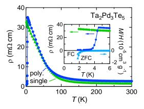
Fig. 2. Temperature dependence of electrical resistivity of the singlecrystalline and polycrystalline samples of  $Ta_2Pd_3Te_5$ . For the single crystal data, electric current was applied parallel to the *b*-axis. The inset shows an enlarged view of the main panel and the temperature dependence of the zero-field-cooled and field-cooled magnetization of the  $Ta_2Pd_3Te_5$  polycrystalline sample measured under a magnetic field of 20 Oe.
