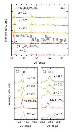
Supplementary Fig. 3. Powder XRD patterns (a) and those around the 200 (b) and 600 (c) reflection peaks of the  $(Nb_{1-x}Ti_x)_2Pd_3Te_5$  (x = 0.1, 0.2, and 0.3) and  $(Nb_{1-y}W_y)_2Pd_3Te_5$  (y = 0.1) polycrystalline samples measured at room temperature. The data of the undoped Nb<sub>2</sub>Pd<sub>3</sub>Te<sub>5</sub> presented in Fig. 1(c) are also shown as a reference. The peak indicated by the triangle is that of an unknown impurity.
