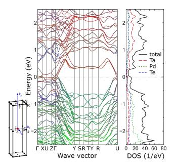
Fig. 5. The electronic states of  $Ta_2Pd_3Te_5$  without spin-orbit coupling. The electronic band structure (left) and total and partial electronic DOS (right) are shown. The Fermi level is set to 0 eV. The first Brillouin zone is shown in the lower left.
