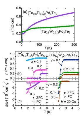
Supplementary Fig. 4. (a) Temperature dependence of the electrical resistivity of the  $(Ta_{0.8}Ti_{0.2})_2Pd_3Te_5$  and  $(Ta_{0.8}W_{0.2})_2Pd_3Te_5$  polycrystalline samples. (b,c) Temperature dependences of the electrical resistivity and zero-field-cooled and field-cooled magnetization of the  $(Ta_{1-x}Ti_x)_2Pd_3Te_5$  (left) and  $(Ta_{1-y}W_y)_2Pd_3Te_5$  (right) polycrystalline samples, respectively. Magnetization was measured under a magnetic field of 20 Oe.
