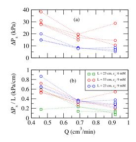
FIG. 3. Variation of (a) saturated pressure drop  $(\Delta P_s)$  with flow rate in a tube of diameter (D = 0.1 cm) and salt concentration  $(c_s = 9 \text{ mM})$  for two different tube lengths and (b) Variation of  $\Delta P_s/L$  with flow rate in a tube of diameter (D = 0.1 cm) and two salt concentrations and tube lengths.
