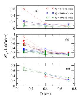
FIG. 4. (a) Variation of saturated pressure drop per unit length  $(\Delta P_s/L)$  with tube diameter (D) for three flow rates (Q). Panels (a), (b) and (c) represent, respectively, data obtained for salt concentrations,  $c_s = 6$  mM,  $c_s = 9$  mM and  $c_s = 12$  mM. Open circles represent data for L = 23 cm, filled circles represent data for L = 53 cm, open squares and diamonds represent data for L = 15.5 cms and filed squares and diamonds represent data for L = 30 cm.
