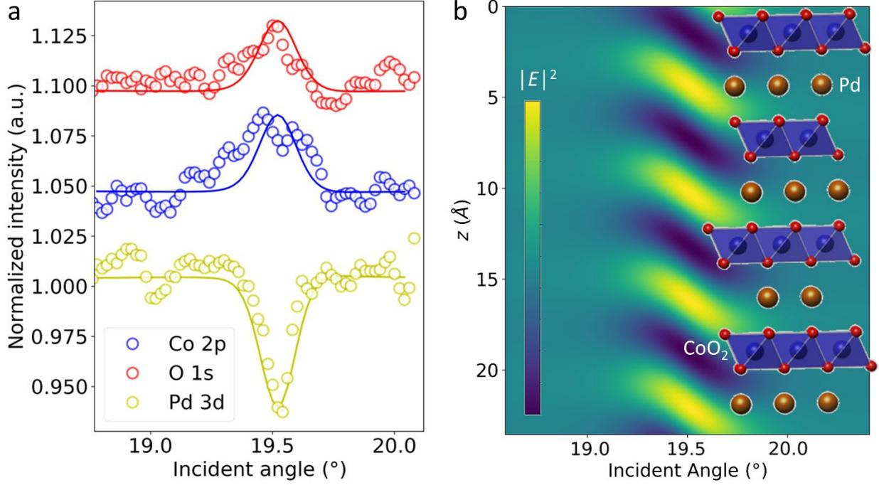
Figure 3: Experimental and simulated rocking curves of core-level spectra of PdCoO<sub>2</sub>. (a) Rocking curves of Pd 3d, Co 2p and O 1s near the (0003) Bragg peak. Experimental data points are shown by circles while the lines are simulated rocking curves obtained from dynamical diffraction theory. (b) Calculated electrical field strength ( $|E|^2$ ) as a function of depth and incident angle.
