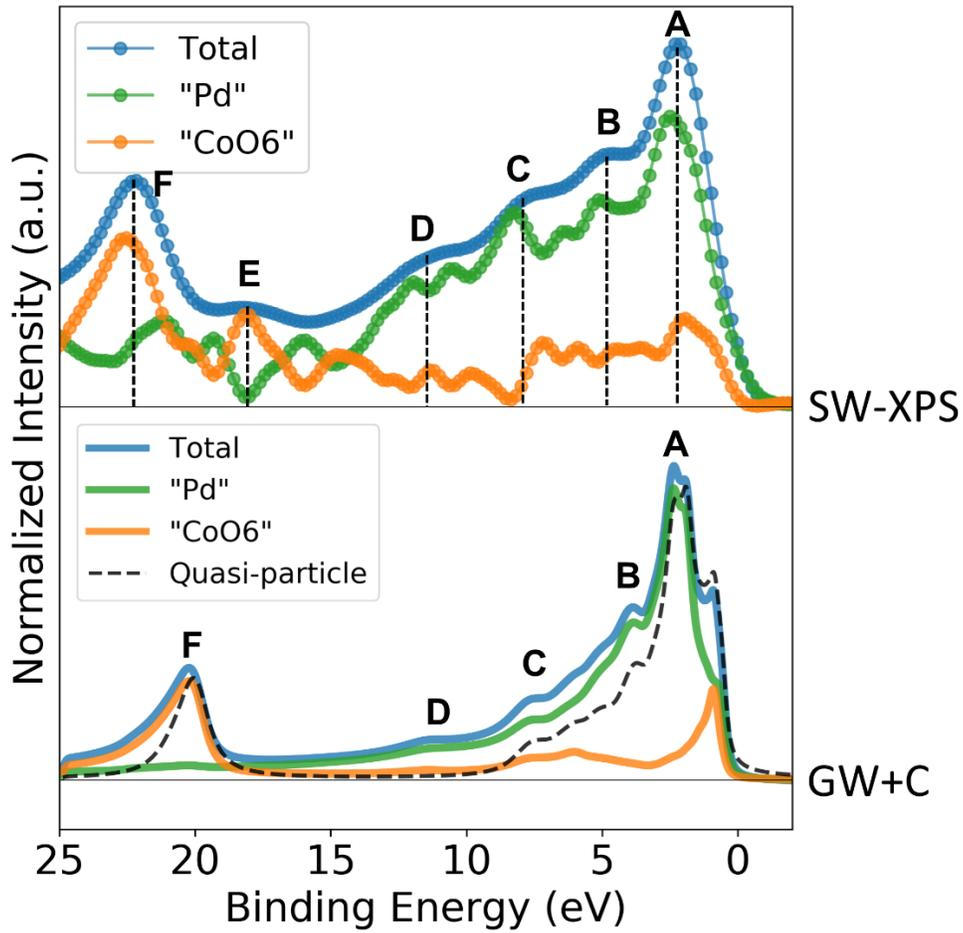
Figure 4: Layer-resolved valence band contributions of PdCoO<sub>2</sub> from standing wave X-ray photoemission spectroscopy (top panel) and GW+cumulant theory calculations (bottom panel). The dashed lines indicate the positions of the peaks in the experimental valence band spectrum.
