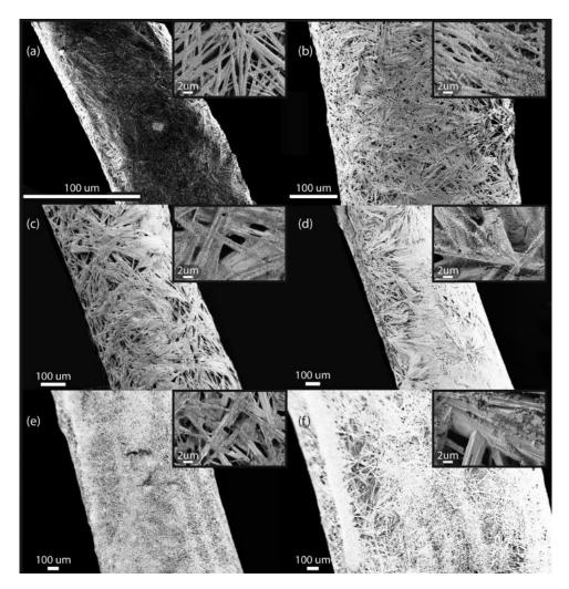
**Figure 2**. SEM images of microcrystalline MAPbI3 deposits on cylinder-shaped quartz substrates with varying diameters: (a) 80  $\mu$ m, (b) 330  $\mu$ m, (c) 400  $\mu$ m, (d) 700  $\mu$ m, (e) 1100  $\mu$ m, and (f) 1800  $\mu$ m. The insets show the magnified image of the deposits on the same size rods as the main figure.
