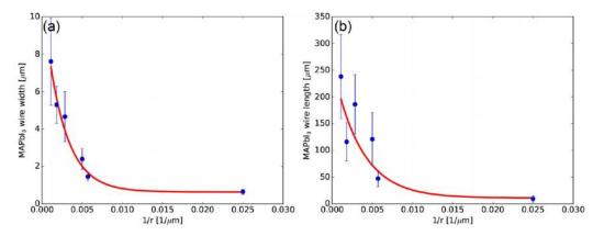
**Figure 3**. Average characteristic sizes of MAPbI3 microwires plotted as a function of the substrate curvature (1/r): (a) average widths and (b) average lengths. The solid line corresponds to the fit with an exponential function.
