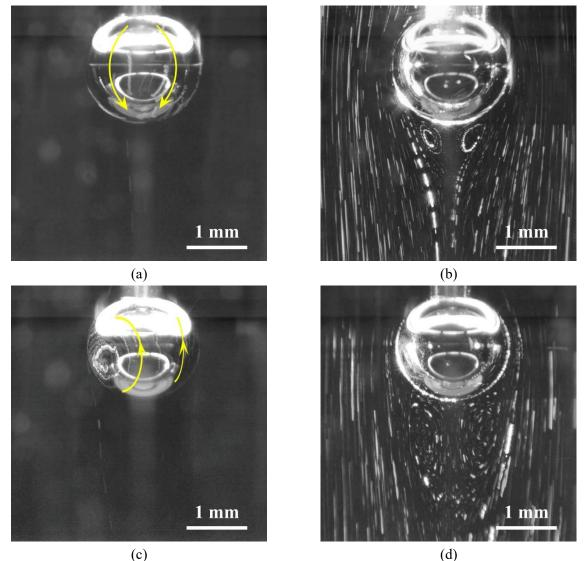
**Figure 6.** Flow structure on the bubble surface in diffuse light (a, c) and around it in laser beam (b, d) in water with Reynolds number 30 (a, b) and 80 (c, d).
