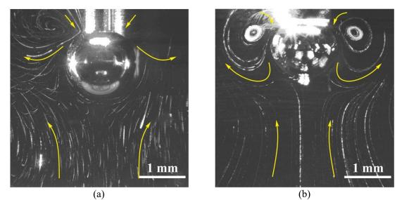
Figure 5. Structures of the thermocapillary flow around the bubble in water (a) and in isopropanol (b).
