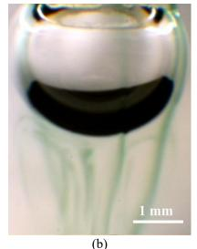
Figure 3. Liquid flow patterns obtained by ejection of dye Reynolds number: 60 (a) and 120 (b).
