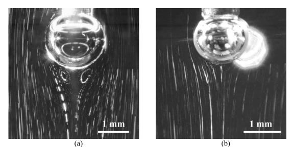
Figure 4. Plan view of the axisymmetric liquid flow around a gas bubble in water (a) and isopropanol (b) with Reynolds number 30.
