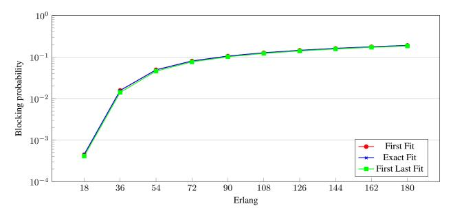
Figure 2: Simulations performed with 3 routes, all conections with BPSK modulation format and not considering optical reach
