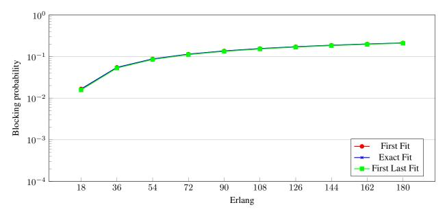
Figure 1: Simulations performed with 1 route, all conections with BPSK modulation format and not considering optical reach
