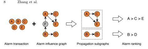
Fig. 3. Processing flow from alarm transaction to ranked alarms.
