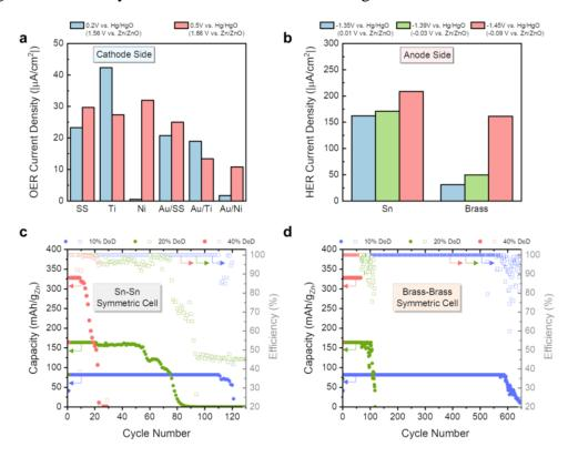
**Figure 2** | **Current collector gas evolution.** Gassing currents after 2 minutes of chronoamperometry for OER at cathode relevant potentials (a) and HER at anode relevant potentials (b). Anode symmetric cell cycling performances with Sn current collectors (c) and brass current collectors (d).
