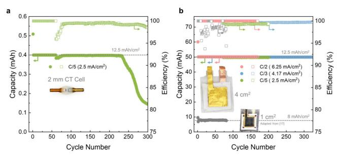
**Figure 6** | **Cycle life performance.** Electrochemical cycle life of (a) 2 mm diameter *in-situ* Au/Ni-Brass CT cell and (b) larger 4 cm<sup>2</sup> Au/Ni-Cu cell and 1 cm<sup>2</sup> cell adapted from [17] with unoptimized current collectors.
