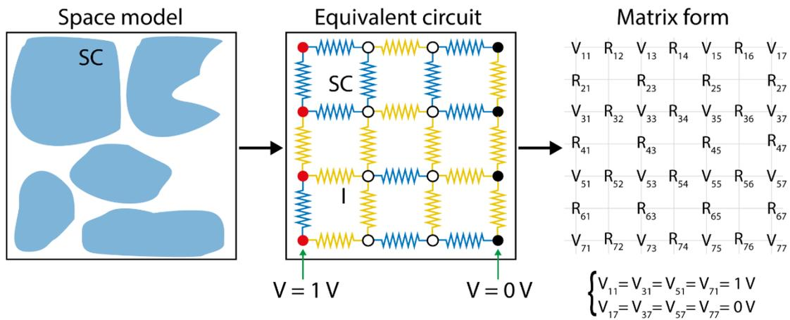
**Figure S5:** Illustration of the NbSe<sub>2</sub> percolative film as a network, (left) random network of superconducting particles, (center) random resistance network derived from the space model, (right) matrix form of the network used to solve the unknown voltages and the currents flowing through each resistor.
