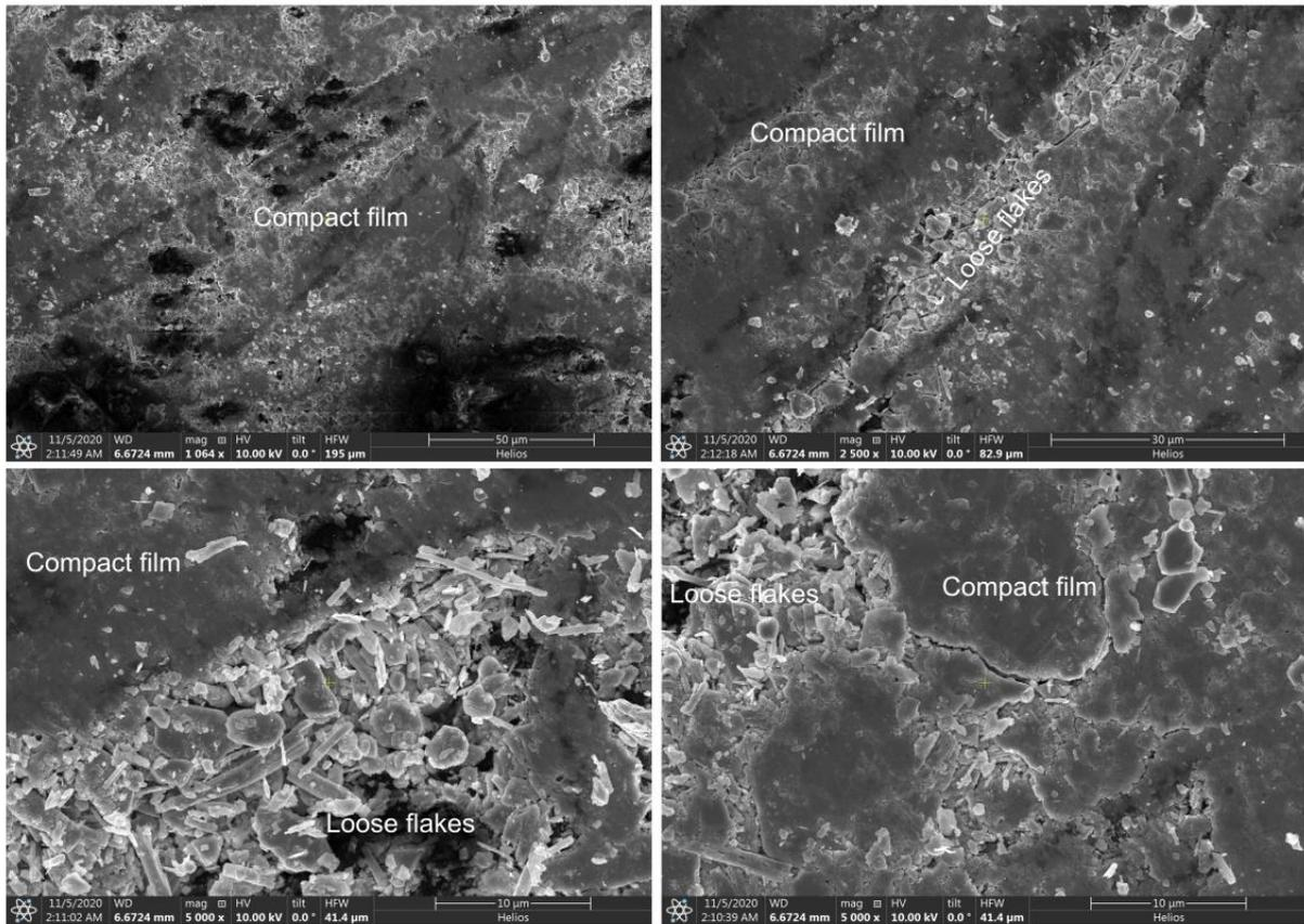
**Figure S3:** More scanning electron microscopy (SEM) images, at different magnifications, acquired on the NbSe<sub>2</sub> film on paper shown in Figure 1 of the main text. The overall film is formed by crushed NbSe<sub>2</sub> flakes that form a compact layer but in some of the gaps between paper fibers one can still observe loose NbSe<sub>2</sub> flakes.
