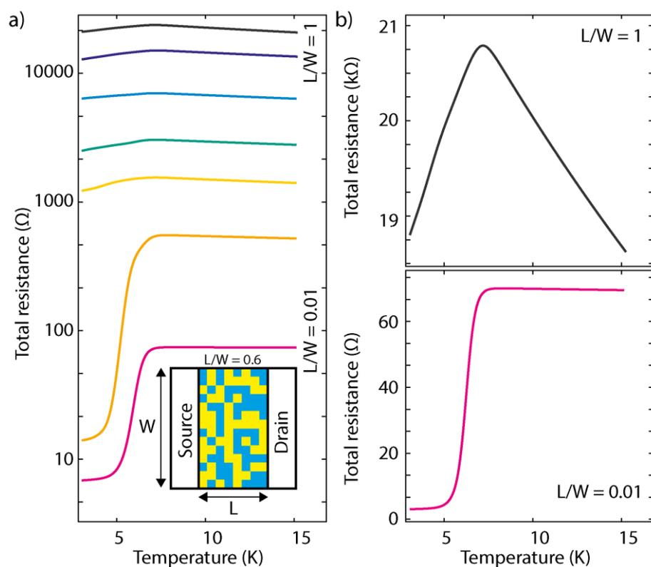
**Figure S8:** a) Semilogarithmic representation of the total resistance of random resistors networks (size  $120 \times 120$ ,  $p = 0.65$ ) as a function of the temperature calculated for different values of the aspect ratio  $L/W$  (where  $L$  is the channel length and  $W$  the width, see inset for an example with  $L/W = 0.6$ ). b) Resistance versus temperature curves for a square channel ( $L/W = 1$ , top) and for a small aspect ratio channel ( $L/W = 0.01$ , bottom).
