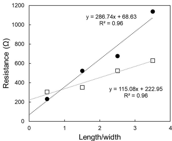
**Figure S1.** Transfer length characterization of two NbSe<sub>2</sub> films on paper to estimate the sheet resistance.
