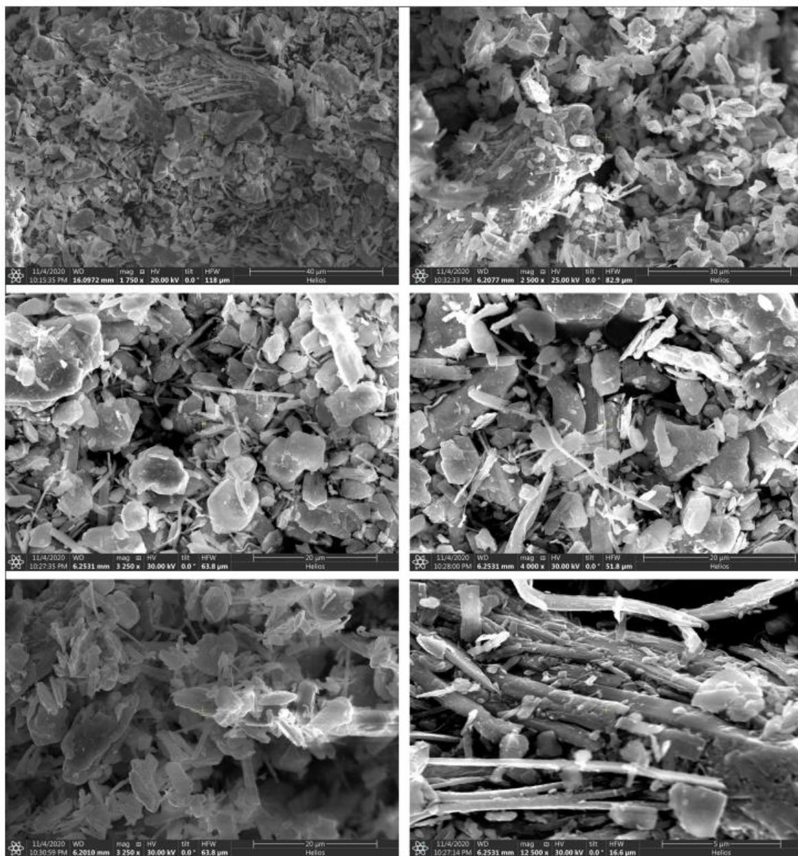
**Figure S2:** Scanning electron microscopy (SEM) images acquired on the NbSe<sub>2</sub> powder source material with different magnifications.
