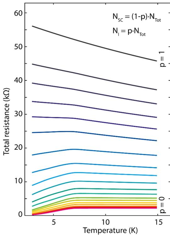
**Figure S7:** Total resistance of random resistors networks (size 120x120) as a function of the temperature and for different amount of superconducting elements in the film. Going from  $p=0$  corresponding to a network entirely made of superconducting elements, to  $p=1$  where the network is fully insulating. The network used in Figure 4 of the main text has  $p=0.65$ .
