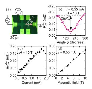
FIG. 2. (a) Microscope image of a Hall bar with Ti/Au electrodes together with the measurement geometry. The angle between the current (I) direction and in-plane magnetic field
