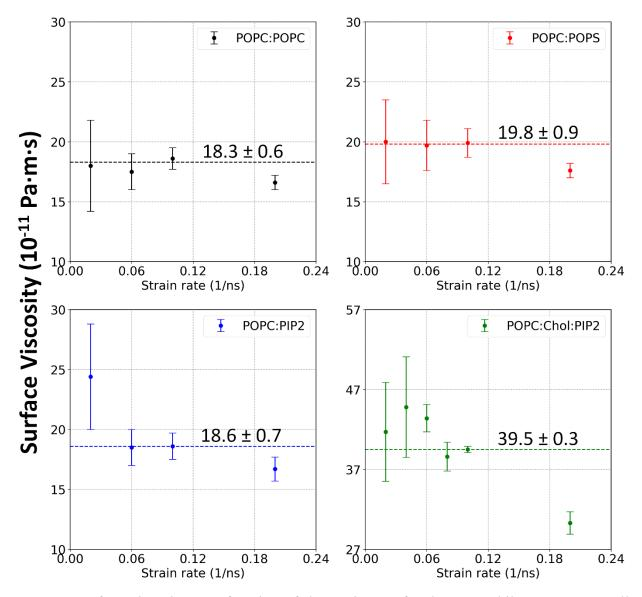
**Figure 5.** Surface viscosity as a function of the strain rate for three C36 bilayer systems. All systems were equilibrated independently to zero surface tension before shearing. Dotted lines show the result of taking inverse-variance weighted averages for strain rates between 0.06 ns<sup>-1</sup> and 0.1
