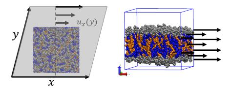
**Figure 2**. Shear deformation for symmetric POPC system. The left plot shows the shear flows along *x*-axis with gradient along *y*-axis, thus achieving the perpendicular shear flow. The right plot shows the flow gradient from the *xz*-plane view. The head groups of bilayers are shown in silver, one hydrophobic chain (C21-C218) of POPC bilayer is shown in blue, and the other chain (C31-C316) is shown in orange VDW mode (hydrogen atoms not shown).
