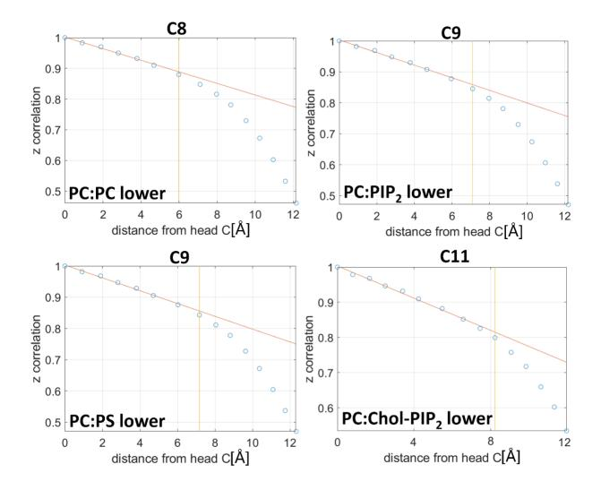
**Figure S2**. Correlation analysis of the lipid height fluctuation between acyl-chain carbons. For each system, *x*-axis stands for the distance between each acyl-chain carbon and the reference carbon C2; *y*-axis stands for the correlation values. The red line shows the best-fit line. The yellow line marks the first point outside of the linear regime that is used to extract the leaflet thickness fluctuations: C8 for PC:PC, C9 for PC:PS and PC:PIP<sub>2</sub>, C11 for PC:Chol-PIP<sub>2</sub>.
