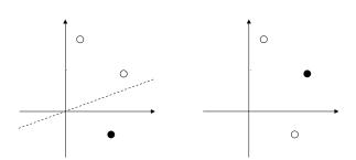
**Figure 1.** Two colorings of three points in two dimensions. In the left one black and white points can be separated by a line through the origin; this coloring therefore represents a dichotomy. For the right one no such separating line exists.
