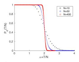
**Figure 2.** Probability  $P_d(T, N)$  that *T* randomly colored points in general position in *N*-dimensional space form a dichotomy as function of the ratio  $\alpha$  between *T* and *N* for different values of *N*. The transition between the limiting values P = 1 at  $\alpha = 1$  and P = 0 at large  $\alpha$  becomes increasingly sharp when *N* grows.
