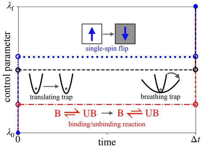
FIG. 1: Short-time efficient protocols (STEPs) for a single spin in a time-dependent magnetic field (blue dots), Brownian particle in a translating harmonic potential (black dashed), Brownian particle in a harmonic potential with time-dependent stiffness (black dashed), and a two-state binding/unbinding reaction system with variable binding and unbinding rates controlled by the chemical-potential difference (red dash-dotted).
