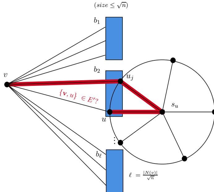
Figure 1: Illustration for the local construction of the 3-spanner. On query  $\{v, u\}$ , namely when querying whether the edge  $\{v, u\}$  belongs to the spanner, the algorithm returns NO since the vertex  $u_j$  is in the same bucket as  $u$  and  $\{v, u_j\}$  is the edge that has minimum rank amongst the edges in the bucket that are incident to the cluster of  $u$ .
