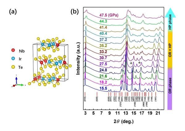
Figure 3. (a) Schematic crystal structure of NbIrTe<sub>4</sub>. (b) X-ray diffraction patterns collected at different pressures. In the range of 15-27 GPa, the sample remains OR phase (see violet regime), while, in the range of 27.5-40.4 GPa, it hosts a mixed phase composed of OR and HP phases (see the orange regime). Upon further compression, the sample possesses a pure HP phase (see the cyan regime).
