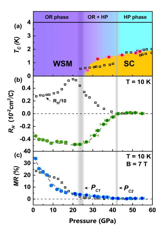
Figure 4. Summary of experimental results of NbIrTe<sub>4</sub> and comparison with TaIrTe<sub>4</sub>. (a) Pressure  $-T_c$  phase diagram with structure information. The data of TaIrTe<sub>4</sub> (see black squares taken from Ref. 31) is included. WSM and SC represent Weyl semimetal and superconducting states, respectively. (b) Pressure dependence of Hall coefficient ( $R_H$ )
