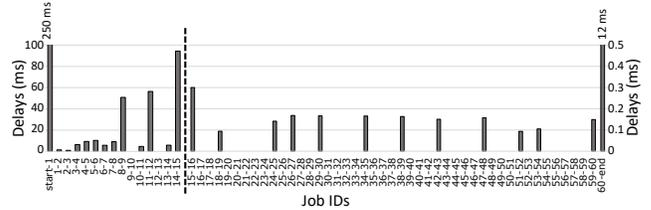
**Figure 5: Intervals between CPU/GPU interactions, accumulated by GPU job. Intervals among earlier jobs are longer than later ones. Workload: AlexNet inference. ACL [22] on Mali G71. Excluded: GPU busy time; parameters loading IO**
