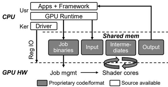
Figure 2: The software/hardware for an integrated GPU
