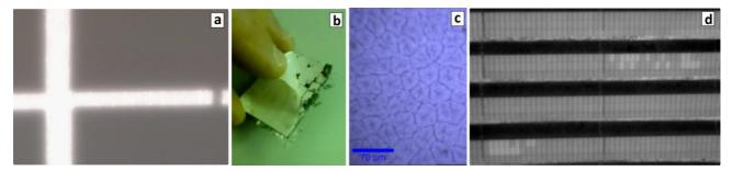
**Figure 6** (a) Photograph of a PV-module with a primer-based SF-type BS taken in transmitted solar light. (b) Photographs of a cut section of a discarded PV-module with a primer-based SF-BS showing signs of drastic degradation of the inner polyolefine layer. (c) Microphotograph of the air-side of a SF-BS showing extensive micro-cracking. (d) Aerial thermographic photograph of a section of solar field showing multiple instances of "bridged" PV-modules.
