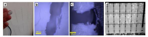
**Figure 5**. (a) Photograph illustrating cracking and "chalking" phenomena typical for PA-BSs. (b,c) microphotographs of a crack in a PA-BS take from the air-side (b) and BS cross-section (c). (d) Aerial thermographic image of a table section with PID-affected PV-modules with PA-BSs.
