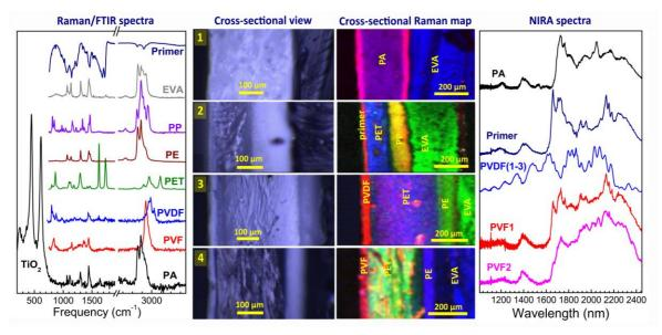
**Figure 2**. Left section - Raman spectra of typical components of BS cross-sections as well as FTIR spectrum of primer air-side (left). *Note*: rutile range is not shown for PVF, PVDF, PP, and PE. Middle section - cross-sectional optical images and multi-spectral Raman maps for different air-side materials. Right section - NIRA spectra of some of tested BSs and EVA encapsulant.
