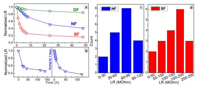
**Figure 3**. (a) Kinetic curves of LR loss during the electrolyte immersion of PV-modules with primerbased SF BS (1), a PA-based NF BS (2), and a DF BS (3). (b) Changes of wet LR for a PV-module NF BS during two cycles of electrolyte immersion interrupted by a 7-day drying pause. (c,d) distributions of wet LRs of PV-modules with NF BSs (c) and SF BSs (d) measured immediately after the electrolyte immersion.
