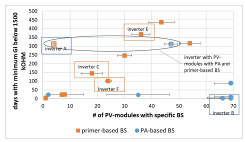
**Figure 8**: Evaluation of GI for inverters with measured and known BS for more than ten PVmodules, error bars visualize the uncertainty of the number of PV-modules due to the varying number of analyzed PV-modules (between 4 and 51 PV-modules per inverter), 2434 days of total operation time.
