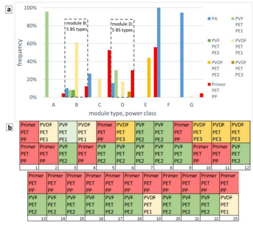
**Figure 4**. (a) Distribution of BS types over the PV-modules of different power classes. (b) An example of two strings (23 modules in each) showing the extreme versatility of BS types for PV-modules type D.
