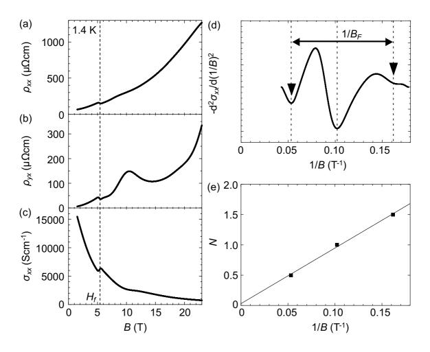
**Figure S2.** SdH oscillation for Gd#4. a) In-plane resistivity  $\rho_{xx}$ , b) Hall resistivity  $\rho_{yx}$ , and c) in-plane conductivity  $\sigma_{xx}$  versus field *B* up to 23 T at 1.4 K.  $H_f$  (= 5.3 T) denotes the spin-flop transition field of the Eu layer. d)  $-d^2\sigma_{xx}/d(1/B)^2$  versus 1/B to estimate the SdH frequency ( $B_F$ ). (e) Landau fan diagram deduced from  $\sigma_{xx}$ .
