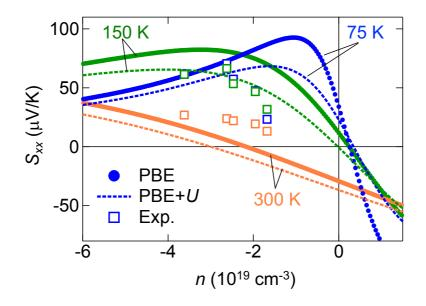
**Figure S5.** Thermopower  $(S_{xx})$  versus carrier density (n) calculated with the PBE and PBE+U methods together with the experimental values (Exp.) shown in Fig. 3(a) in the main text. Spin-orbit coupling is included in transport calculations shown here.
