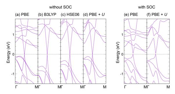
**Figure S4.** The first-principles band structures calculated with (a) PBE, (b) B3LYP, (c) HSE06, and (d) PBE+*U* methods without including the spin-orbit coupling. The band structures calculated including the spin-orbit coupling are also shown for (e) PBE and (f) PBE+*U* methods. For comparison among the different methods, we set the energy zero to be the Dirac point along the  $\Gamma$ -M line for panels (a)-(d) and the valence band top along the  $\Gamma$ -M line for panels (e)-(f).
