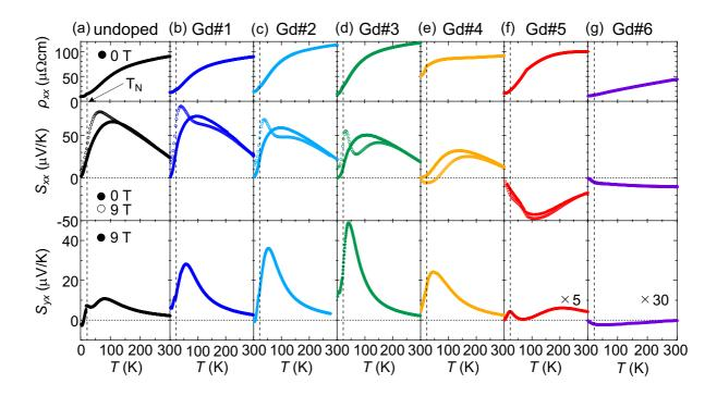
**Figure 2.** Variation of thermoelectric properties upon  $E_F$  for (Eu,Gd)MnBi<sub>2</sub> single crystals. a)-g) In-plane resistivity  $\rho_{xx}$  (top), thermopower  $S_{xx}$  (middle), and Nernst signal  $S_{yx}$  (bottom) versus temperature T. The magneto-thermopower and Nernst signal were measured at 9 T (B||c). A vertical dashed line denotes the antiferromagnetic transition temperature of the Eu layer ( $T_N$ ) for each sample.
