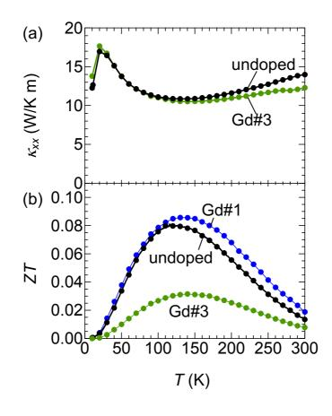
**Figure S3.** Thermoelectric efficiency for hole-doped EuMnBi<sub>2</sub>. Temperature dependence of a) in-plane thermal conductivity  $\kappa_{xx}$  and b) dimensionless figure of merit *ZT*.
