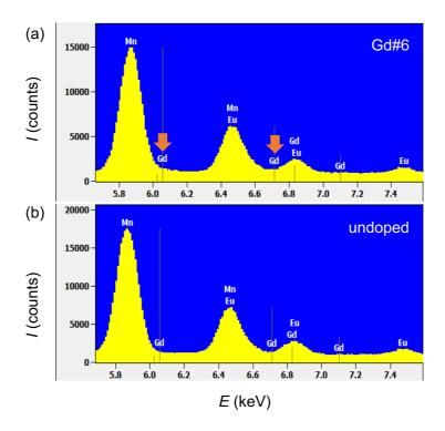
**Figure S1.** Energy dispersive x-ray analysis. The spectra for a) Gd#6 and b) undoped samples are shown. The energy range near the Gd *L* edge is selected.
