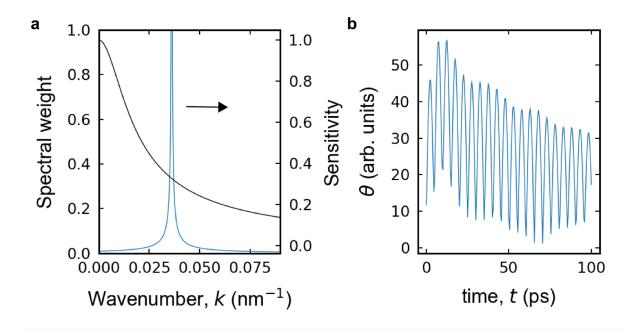
**Figure S2**: a) Wavepacket distribution (black line, left axis) and the sensitivity function as given by the first term of the integrand in Eq. S1.17 (blue line, right axis). b) The resulting time-resolved MOKE signal, given by the wavepacket distribution and the sensitivity function from panel a).
