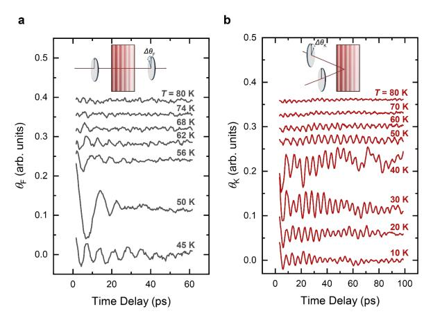
**Extended Data Figure 2: Magnon time traces at different temperatures. a)** Time resolved polarization rotation in the transmission (a) and reflection geometry (b) following excitation at hv = 3.1 eV at different temperatures. The probe incidence angle is near-normal, with  $\lambda = 640$  nm and  $\lambda = 700$  nm for the measurements in panel a and b, respectively.
