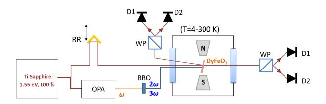
**Extended Data Figure 1: Experimental setup.** RR: gold retroreflector mounted on a motorized precision delay stage, OPA: optical parametric amplifier, BBO:  $\beta$ -barium borate crystal, WP: Wollaston Prism, D1, D2: pair of balanced silicon photodetectors.
