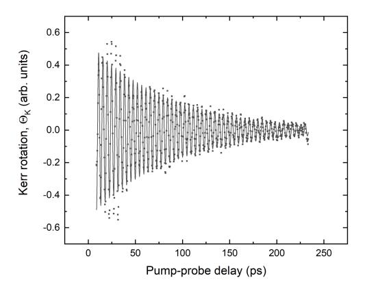
Figure S4: Time-resolved polarization rotation originating from a propagating magnon, as obtained in the reflection geometry. The solid line represents a best fit of a damped sine, giving a lifetime of ~85 ps.
