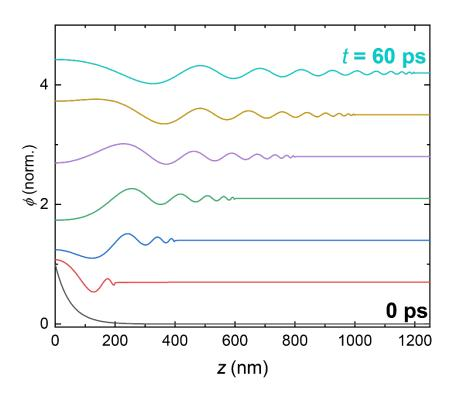
**Extended Data Figure 4: Simulations of the light-induced spin wave dynamics.** Real-space distribution of the magnon spin deflection at different times *t*, after optical excitation at 3.1 eV with a penetration depth of 50 nm, as determined by Eq. (3).
