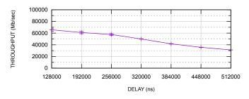
Fig. 2: Throughput results from the BlueField-2 SmartNIC with different delay configurations (8 threads, packet size 10KB, burst 25)
