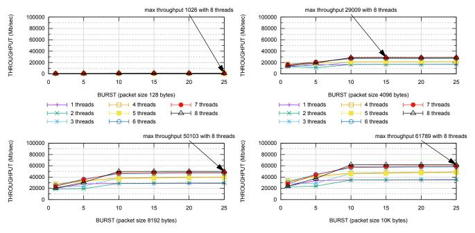
Fig. 1: Throughput results from the BlueField-2 SmartNIC in host separated mode
