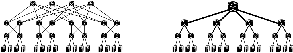
Figure 1: Fat tree topology [1] constructed using f = 4 -port switches (left) and corresponding forwarding abstraction (right).
