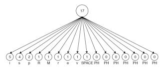
Fig. 2. Fully linked 16-mal Huffman Tree.
