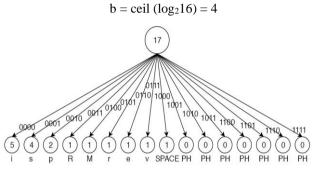
Fig. 3. 16-mal Huffman Tree with binary values assigned to edges.
