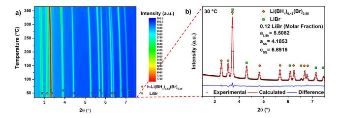
*Figure 1. a)* in situ SR-PXD data for sample s1 heated from RT to 370 °C (heating rate 5 °C/min) in Ar atmosphere. Temperatures have been calibrated using LiBr as internal standard. *b)* Rietveld refinement of sample s1 at 30 °C ( $R_{wp}$  3.23 %). Values of lattice constants for LiBr and hexagonal solid solution (SS) are reported in Å.
