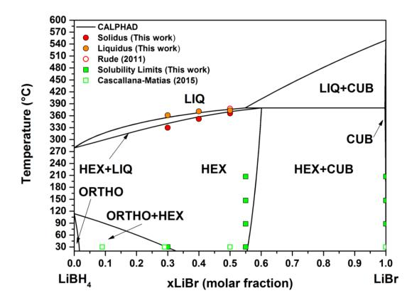
*Figure 5. Lines: assessed phase diagram for the* LiBH<sub>4</sub>–LiBr system. Orange circles: experimental liquidus data from this work; red-open circle: liquidus temperature from ref.<sup>18</sup>; red circles: experimental liquidus data from this work; green squares: experimental solubility limits from this work; green-open square: literature solubility limit from ref.<sup>14</sup>.
