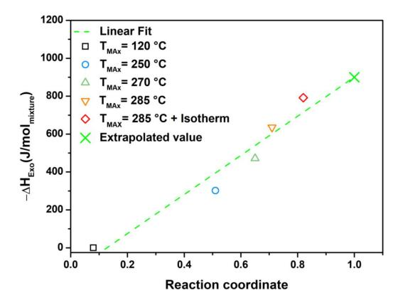
**Figure 4.**  $\Delta H_{Exo}$  measured by DSC as a function of the reaction coordinate for the formation of the LiBH<sub>4</sub>-LiBr hexagonal solid solution in s5.
