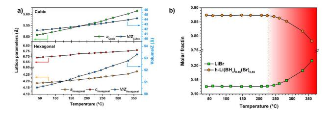
*Figure 2. a)* Lattice parameters and unit cell volume (V/Z) as a function of temperature for h-Li(BH<sub>4</sub>)<sub>1-x</sub>(Br)<sub>x</sub> hexagonal solid solution and cubic LiBr. *b*) Molar phase fraction of h-Li(BH<sub>4</sub>)<sub>1-x</sub>(Br)<sub>x</sub> hexagonal solid solution and cubic LiBr as a function of temperature.
