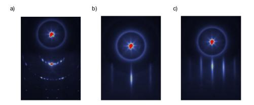
**Figure S1** Reflective High Energy Electron Diffraction (RHEED) pattern obtained at 15kV, 1.5A. a) Clean Si (111) substrate showing 7x7 surface reconstruction before growth. b) RHEED of MBT/BT/MBT heterostructure taken after growth along  $[11\overline{2}]$  direction and c) taken along [110] direction. The sharp high intensity streaks in the patterns indicate large area of single-crystal epitaxial thin films.
