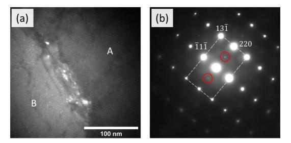
Figure A. 1: (a) dark-field image from  $\gamma'$  reflections at a grain boundary in the as-built microstructure. (b)  $[1\overline{1}\overline{2}]$  zone axis diffraction pattern acquired in grain A. The red circles denote the 110 reflections associated with the  $\gamma'$  phase.
