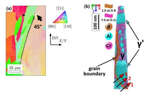
Figure 8: (a) BF-IPF map of the heat-treated microstructure showing in arrow the uncracked region of the partially cracked grain boundary selected for APT. (b) Atom probe reconstruction of a specimen including the grain boundary, displayed with 1.5 at.% and the  $\gamma$ ' particles.
