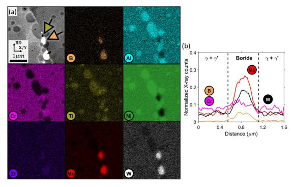
Figure 5: (a) BSE contrast image of the heat-treated microstructure near a grain boundary and corresponding X-ray maps. The colour contrast is proportional to the number of X-rays counted for each element. (b) X-ray count profile across a boride. The X-ray counts associated to each elements are normalized by the total number of counts at each position along the profile.
