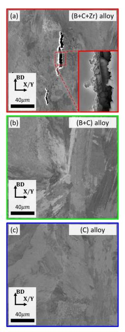
Figure 1: SEM-SE contrast micrographs of the as-built microstructure of (a) the (B+C+Zr) alloy, (b) the (B+C) alloy, (c) the (C) alloy. An enlarged view of the crack surface is shown in (a). The enlarged view was acquired with an in-lens detector.
