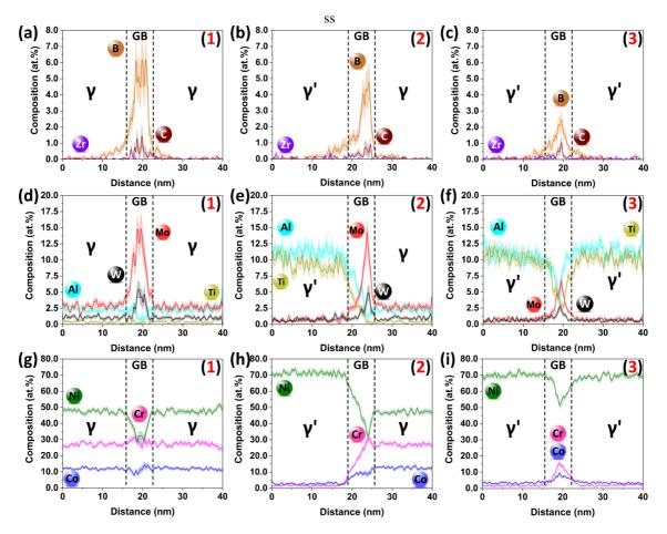
Figure 9: Composition profiles across the grain boundary taken from the heat-treated microstructure for a  $(\gamma - \gamma)$  interface, a  $(\gamma' - \gamma)$  interface and a  $(\gamma' - \gamma')$  interface. (a,b,c) boron, carbon and zirconium. (d,e,f) aluminium, titanium, molybdenum and tungsten. (g,h,i) chromium, nickel and cobalt. The number on each figure corresponds to the profile location denoted by arrows in Figure 8b.
