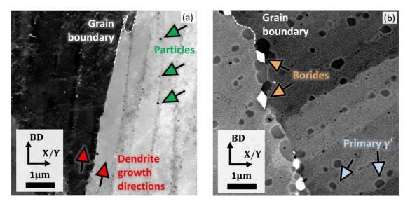
Figure 4: BSE contrast images of (a) the as-built microstructure, (b) the heat-treated microstructure.
