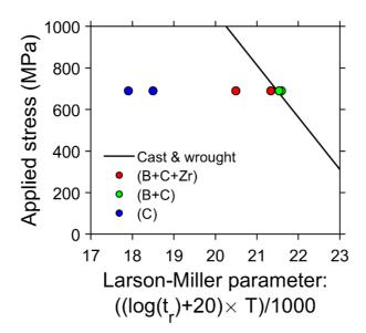
Figure 2: Creep resistance of the heat-treated samples plotted in terms of Larson-Miller parameter. The behaviour of cast & wrought  $AD730^{\circ\circ}$  is shown as a line for comparison. The grain size of the cast & wrought alloy is 10 in ASTM standard [29], which corresponds to a diameter of 11.2µm according to conversion tables.
