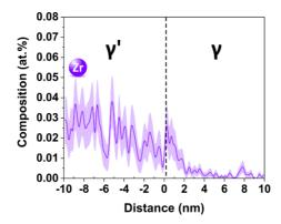
Figure 10: Zirconium composition profile across a  $\gamma/\gamma'$  interface away from the grain boundary.
