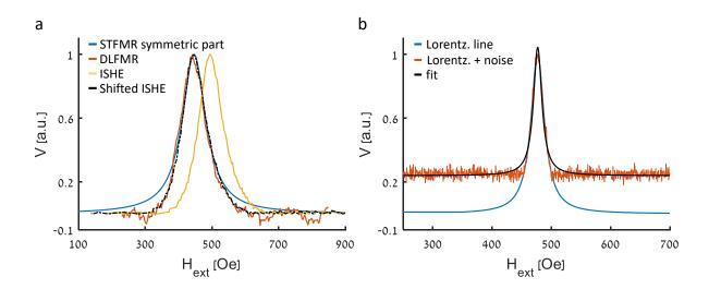
Fig. 4. (a) Symmetric part of the STFMR measurement (blue) together with the responses of the DLFMR (red) and ISHE (yellow) measurements and the shifted ISHE response (dashed black). Traces are normalized to the peak value. (b) Noise simulation. Blue solid line indicates an ideal Lorentzian lineshape. Red solid line illustrates the calculated Lorentzian lineshape together with a simulated noise floor. Black solid line is a fit of the simulated noisy Lorentzian to a noise-free response.
