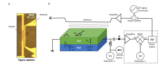
Fig. 1. Experimental setup. (a) Patterned SHE device with a micro-antenna. (b) Schematic of the measurement setup that includes the STFMR, ISHE, and DLFMR.
