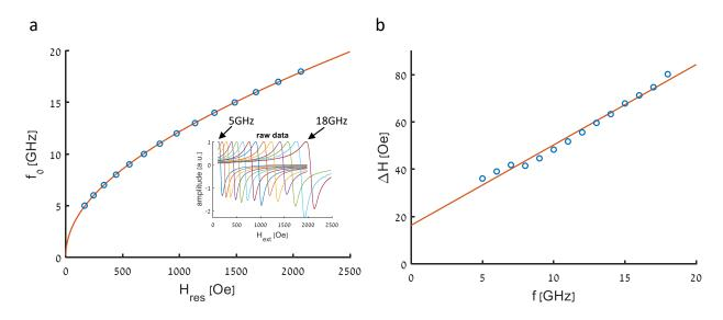
Fig. 2. (a) STFMR Frequency-field dispersion relation. Open blue circles indicate the measurement. Solid red line indicates Kittel's formula. Inset illustrates the measured STFMR responses for 5 - 18 GHz. (b) Resonance linewidth as a function of frequency. Solid red line indicates the linear fit.
