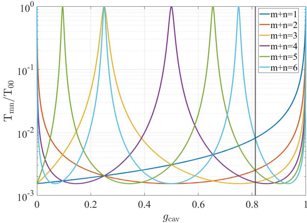
Figure 2 – The expected power transmission for the first 6 higher-order modes (Eq. 1). Finesse is altered until local minimums reach the desired level, which in our case is  $\sim 2$  orders of magnitude. This is achieved as displayed, at  $\mathcal{F} = 40$ . Appropriate local minimums then reveal the acceptable cavity g-factors. The x line shows the specification g-factor.
