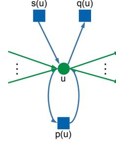
Fig. 2: Cloud-augmented graph for node  $u$ , where  $p(u)$  represents the processing unit that hosts flow processing functions,  $s(u)$  the source unit from which flows enter the cloud network, and  $q(u)$  the demand unit via which flows exit the cloud network.
