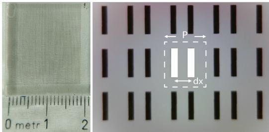
FIG. 1: (a) Photograph of the sample and (b) microscope image of several unit cells of the sample. The period  $P$  and distance between rods  $dx$  are also indicated in the image.
