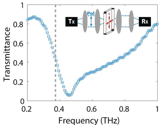
FIG. 3: Measured far-field transmittance spectrum under normal incidence using a THz time-domain spectrometer, as schematically depicted in the inset. The expected frequency of the BIC, as obtained from the CEMD model, is indicated by the grey dashed line. The spectral resolution of the measurements is 7 GHz.
