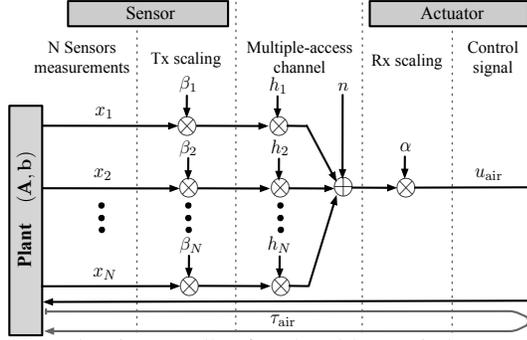
Fig. 1: Over-the-air controller for closed-loop wireless control systems.
