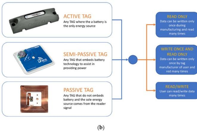
Fig. 2. The three types of RFID technology.
