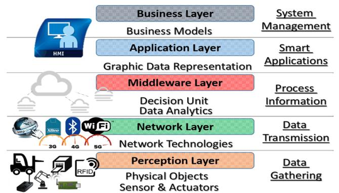
Fig. 6. The five layer model of IoT architecture.
