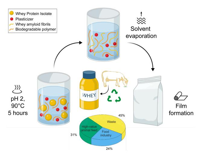
**Figure 1.** Schematic representation of the bioplastic preparation protocol. Each year in Switzerland 1.3 Mt of whey are produced, of which only half of it is valorized efficiently<sup>[16]</sup>. Whey protein isolate, Glycerol, and PVA are dispersed in water, the solution is heated at 90°C for 5 hours to allow β- lactoglobulin monomers to self-assemble into amyloid fibrils. The solution is then cast to obtain bioplastic film through solvent evaporation.
