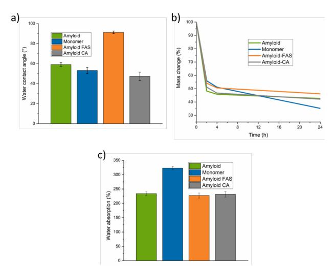
**Figure 3.** a) Water contact angle of the films after different crosslinking treatment. b) mass change, and c) water absorption.
