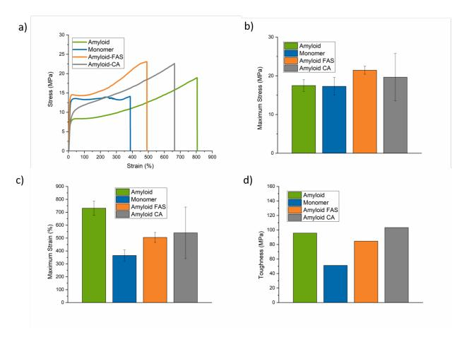
**Figure 4.** Mechanical properties of films. a) stress-strain plot, b) maximum stress, c) maximum strain, and d) toughness.
