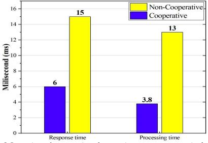
Fig. 2: Processing and response time of cooperative versus non-cooperative fog.
