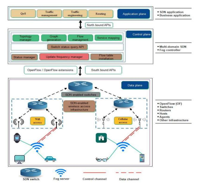
Fig. 1: A simplified view of the SDN-enabled fog computing architecture
