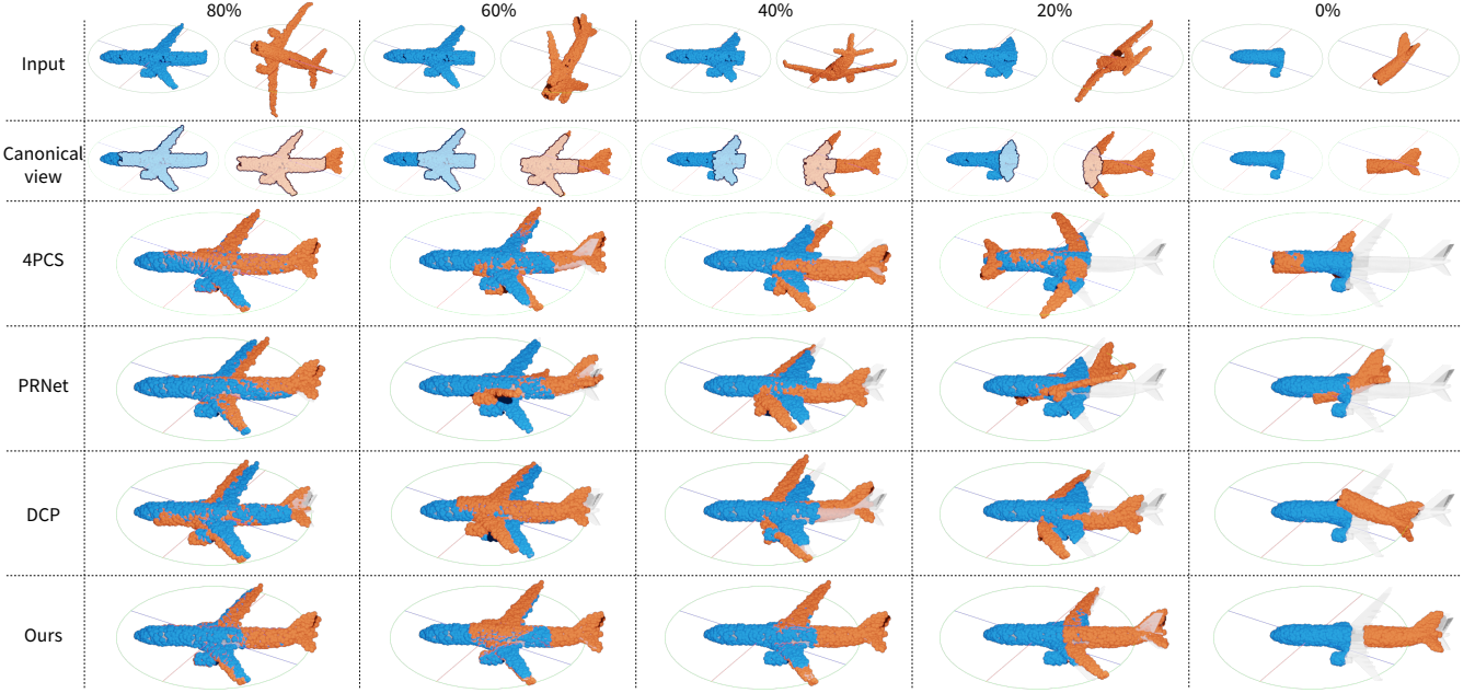
Fig. 8: Visual comparisons of our CTF-Net to other registration methods on different overlap data. The input pair of partial parts is shown in the first row. To better illustrate the overlap region, we show the input pair in the second row after rotating each part into a canonical view, and mark the overlap region with a lighter color. Next four rows show the registration results provided by 4PCS, DCP, PRNet and ours respectively. Here we only show the registration results that takes the blue part as the anchor.
