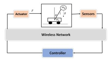
Fig. 1. Inverted pendulum system model.
