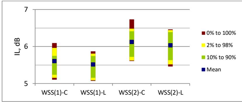
Fig. 3. Measured C + L WSS insertion loss distribution for C and L bands.
