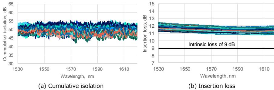
Fig. 4. Measured spectra of  $16 \times 8$  MCS. (a) Cumulative port isolation and (b) insertion loss.
