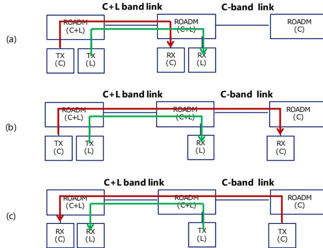
Fig. 7. Network models corresponding to (a) scenario 1, (b) scenario 2, and (c) scenario 3.
