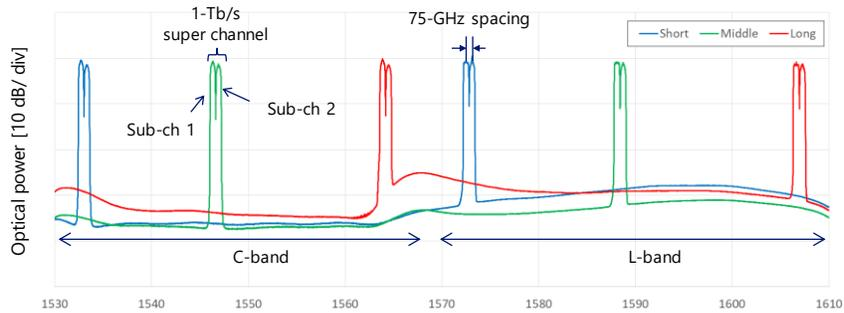
Fig. 6. Test signal spectra. Each spectrum is composed of two subcarriers with 500-Gbps signal.
