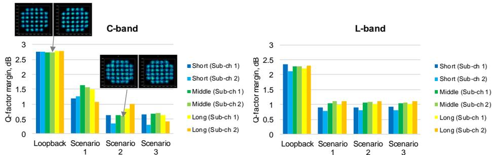
Fig. 8. Q-factor margin from FEC threshold of transponder in the three scenarios for C and L band signals.
