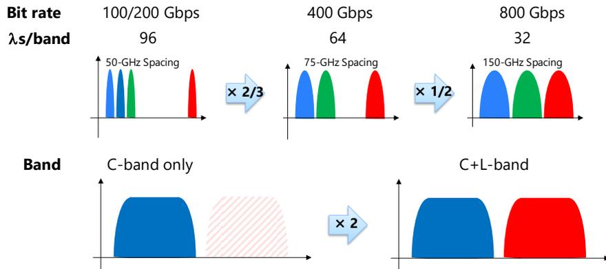
Fig. 1. Impact of higher baud rate signal on the number of WDM channels.
