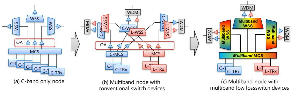
Fig. 2. CDC-ROADM node configuration for (a) C band only, (b) C + L band with conventional switch devices, and (c) C + L band with multiband switch devices.
