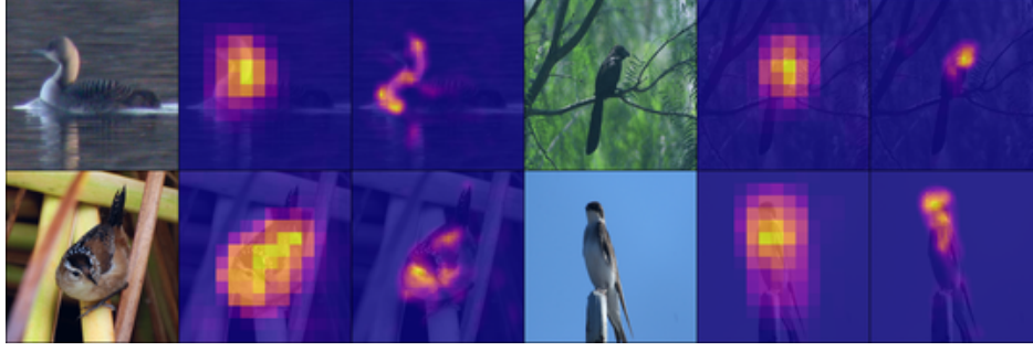
Figure 4: From left to right: original image, attention maps of CNN with lower and then higher-resolution feature maps.
