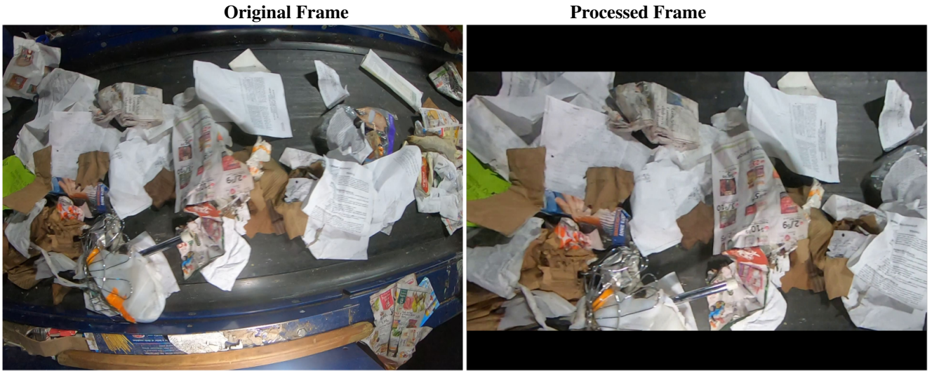
Figure 12. Left: sample video frame from ZeroWaste before collection of target objects to be removed from the conveyor belt. Right: the same video frame processed as described in section 3: fisheye effect removed, frame rotated to make the conveyor belt parallel to the image border, regions outside conveyor belt cropped out, motion blur removed.
