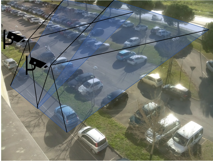
Figure 1: An example of two cameras monitoring the same parking area with partially overlapping fields of views. This redundancy provides robustness and fault-tolerance but also raises the problem of aggregating knowledge extracted from the individual cameras.
