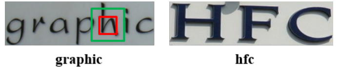
Fig. 6. Two sample images from the ICDAR2003 dataset. In the first example, for recognizing the character “h”, the classical RF (red square) and desired non-classical RF (green) of GRCNN are shown. If the non-classical RF covers unrelated information, such as the characters “p” and “i”, it will distract the model.
