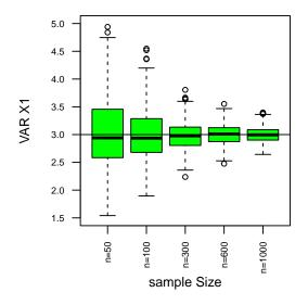
**Figure 5.** Simulation results: bivariate case. Estimates of  $\sigma_{x_1}^2$  for sample sizes of n = 50, 100, 300, 600, 1000, and k = 10 intervals for each variable. The horizontal solid line corresponds to the true value  $\sigma_{x_1}^2 = 3$ .
