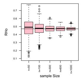
Figure 7. Simulation results: bivariate case. Estimates of  $\rho$  for sample sizes of n = 50, 100, 300, 600, 1000, and k = 10 intervals for each variable. The horizontal solid line corresponds to the true value of  $\rho_{x_1,x_2}$ .
