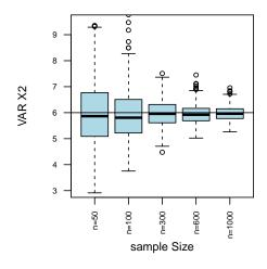
Figure 6. Simulation results: bivariate case. Estimates of  $\sigma_{x_2}^2$  for sample sizes of n = 50, 100, 300, 600, 1000, and k = 10 intervals for each variable. The horizontal solid line corresponds to the true value  $\sigma_{x_2}^2 = 6$ .
