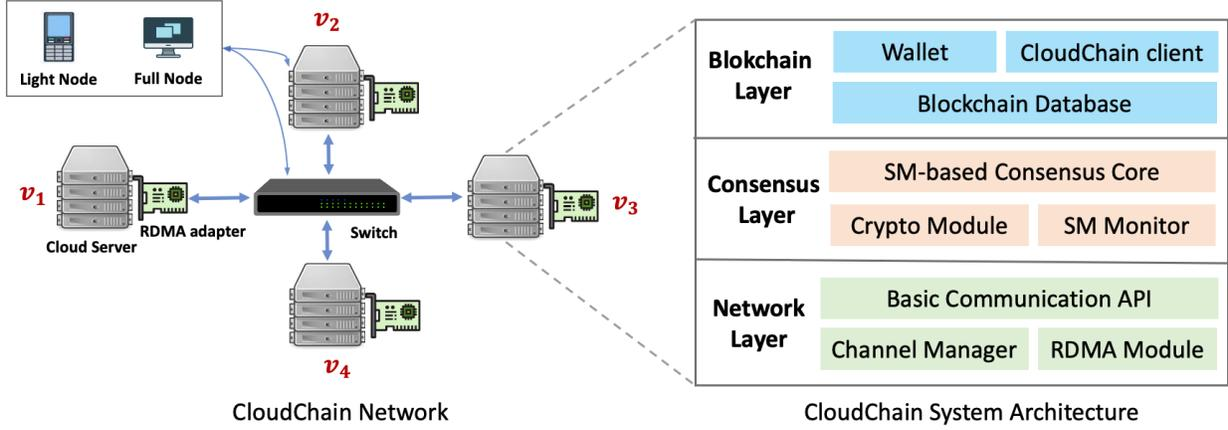
Fig. 3. Network and system architecture of CloudChain
