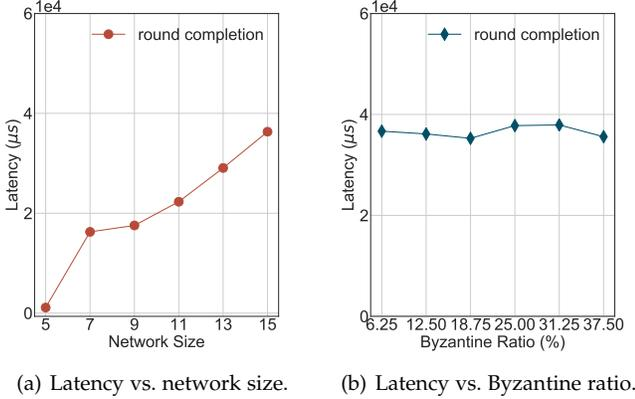
Fig. 7. Latency for the SM-based consensus algorithm.
