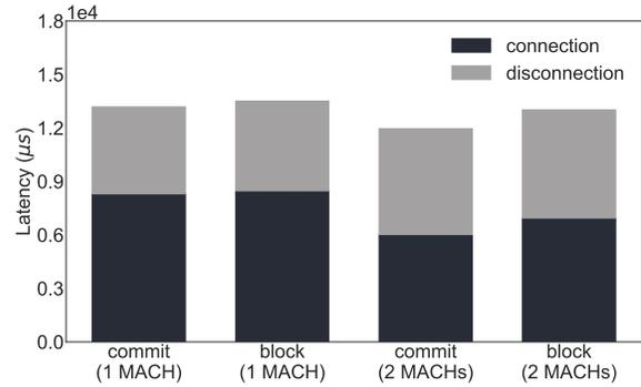
Fig. 4. Latencies for QP connection and disconnection
