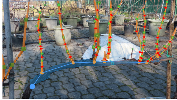
Fig. 4: An output example of potential pruning points generation overlaid on the segmentation output, where blue represents the main cordon class, orange the cane class and green the node class, with the red markers representing the generated potential pruning points.
