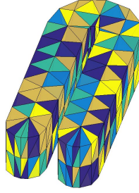
Figure 5.1: An illustration of block CV using a triangulation. Tetrahedra with the same color belong to the same fold.
